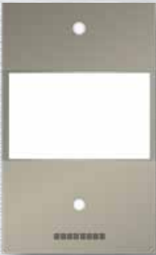
CE-e2 Arch-Shaped Part: Milky-White Acrylic Sheet Flat Panel: Steel Sheet with Color Paint Light: LED (White)+ Downlight(3W, LED) Emergency Light(4.5W, LED) (In case of deep car, the design of ceiling will be changed.)
